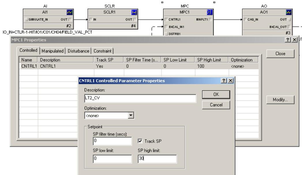
Figure 2.11 Set parameter properties for the MPC variables.
