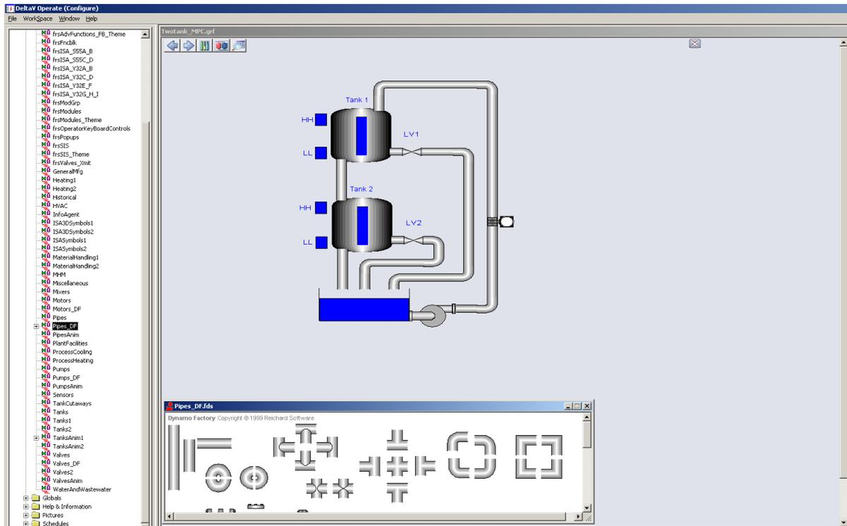
Figure 4.13 Adding a reservoir tank and pipes to the picture interface.
