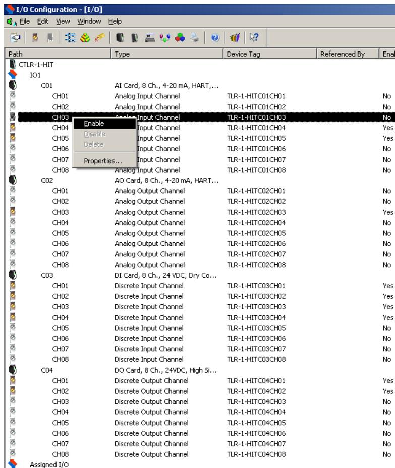
Figure 2.6 Enabling I/O Configuration.
