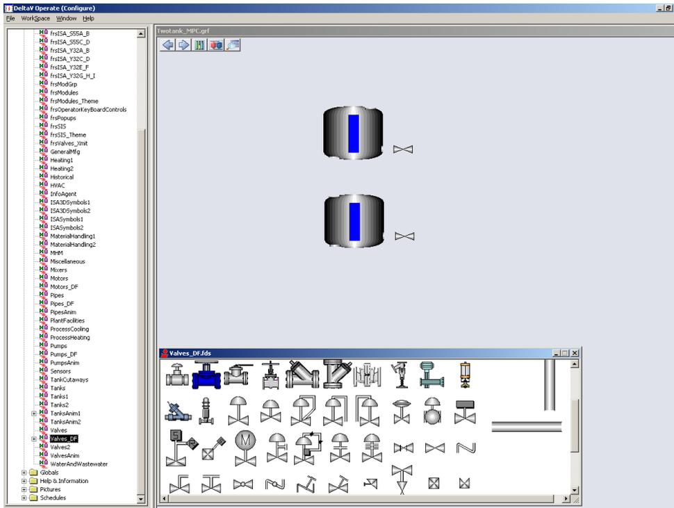
Figure 4.7 Adding valves to the picture interface.
