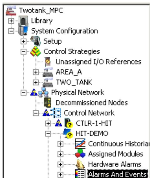
Figure 2.15 Assigning TWO\_TANK area to Alarms and Events and Continuous Historian.
