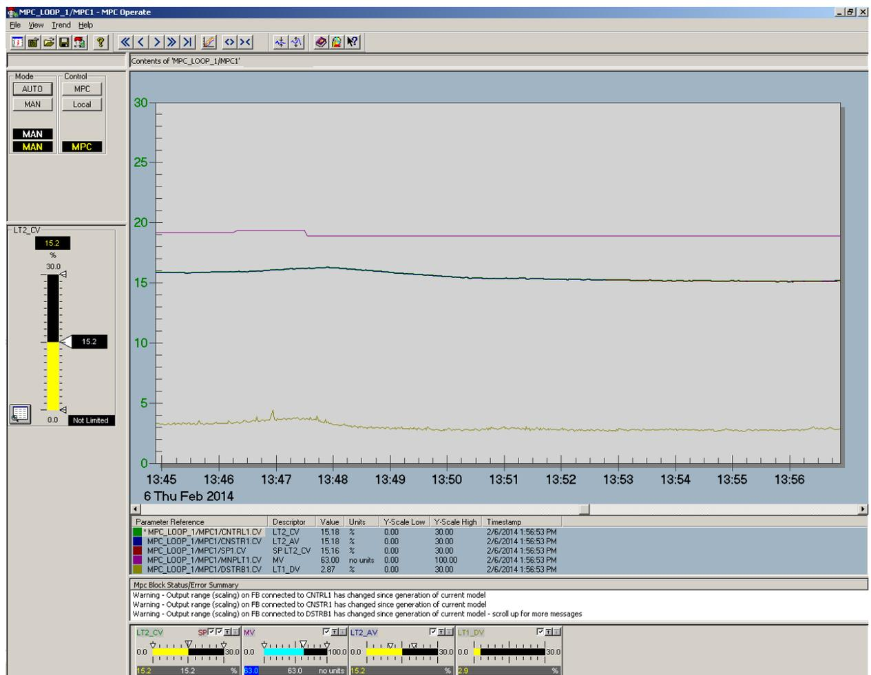
Figure 3.4 Adjusting level manually in MPC Operate.
