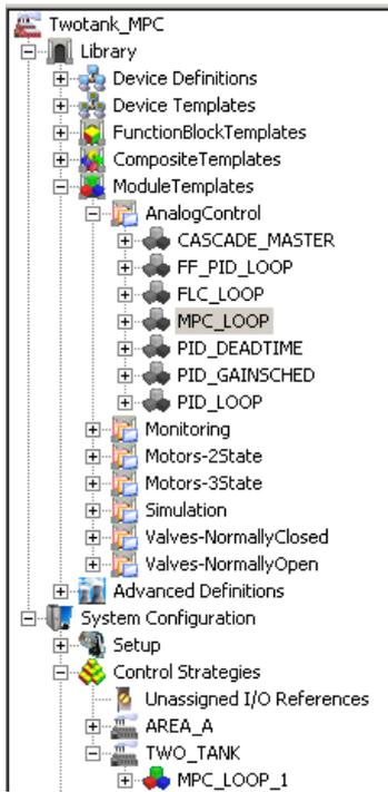
Figure 2.2 Control module MPC\_LOOP\_1 from library.
