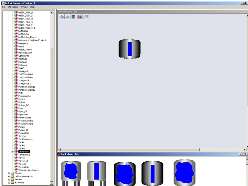
Figure 4.4 Adding a tank to the picture interface.
