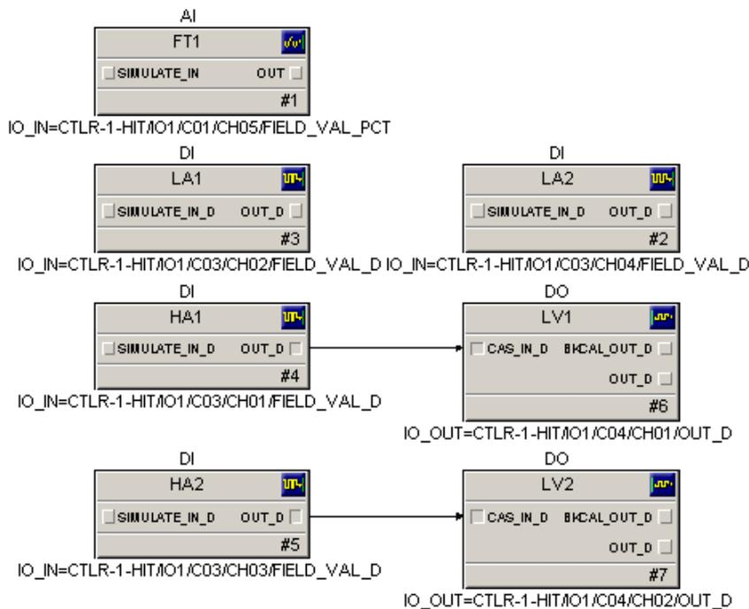
Figure 2.14 Connected and configured Analog- and Digital blocks.
