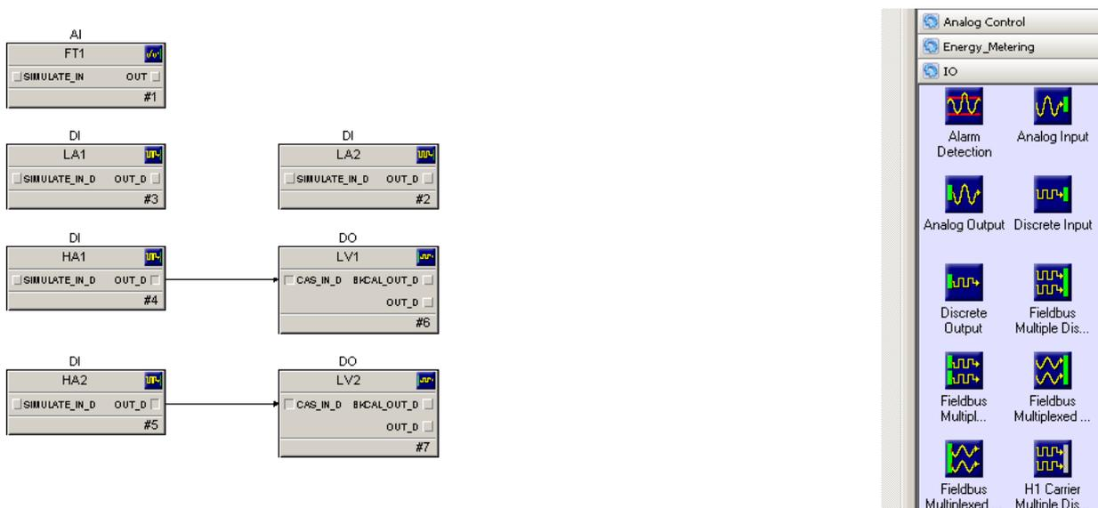
Figure 2.13 Analog- and Digital signal blocks for the physical model.
