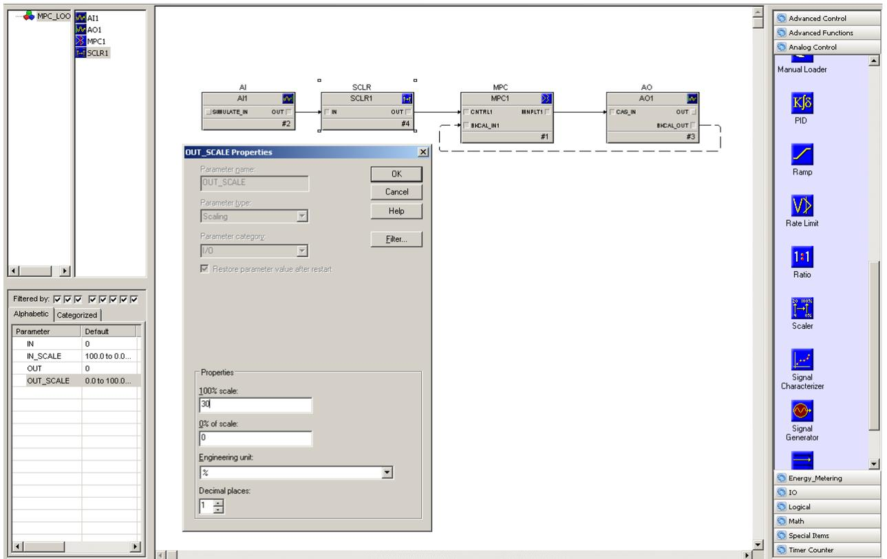
Figure 2.8 Connecting AI and Scaler block to the MPC block.
