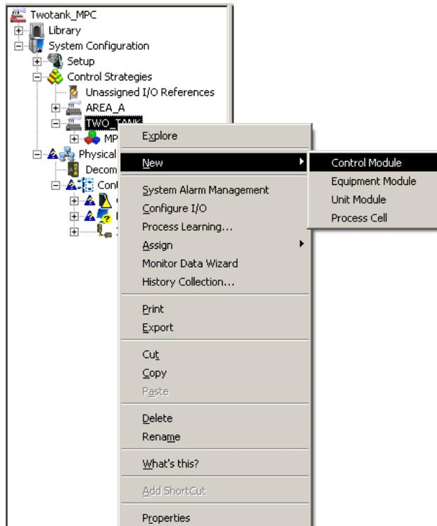
Figure 2.3 Creating a control module for the I/O's.
