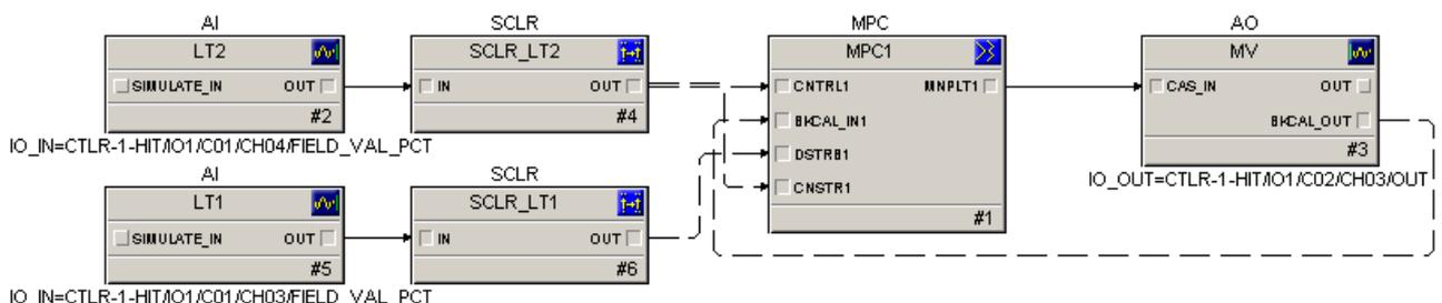
Figure 2.12 Constraint and disturbance parameters connected to the MPC block.
