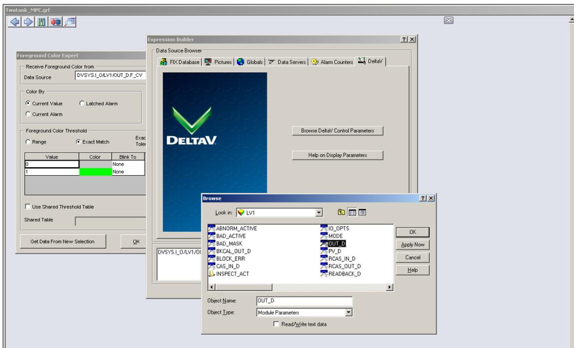
Figure 4.10 Adding datalink to the valve.
