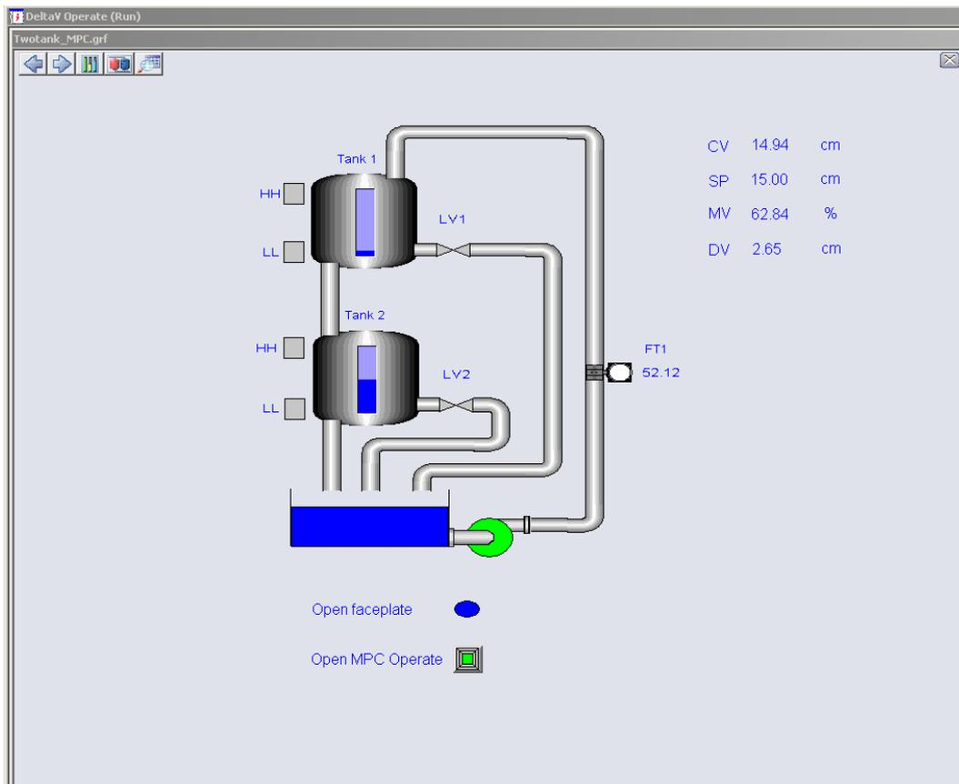
Figure 5.1 Running Level Tank system in DeltaV Operate Run.
