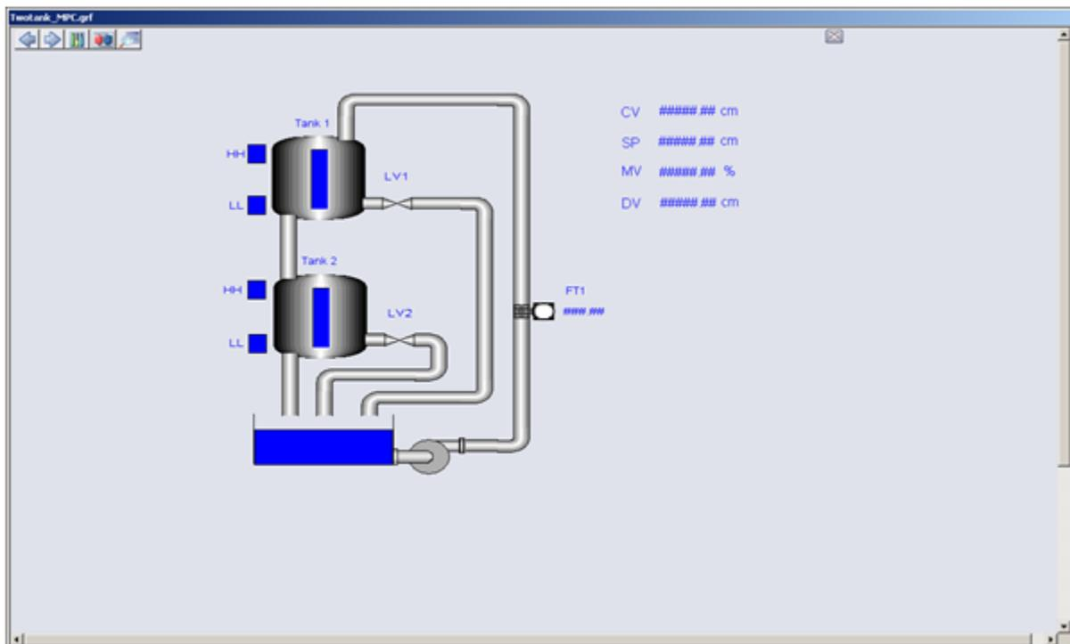
Figure 4.18 Picture interface with added datalinks.
