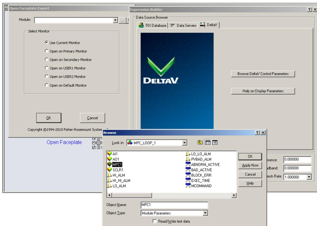
Figure 4.19 Creating a button to open the MPC-controller faceplate.
