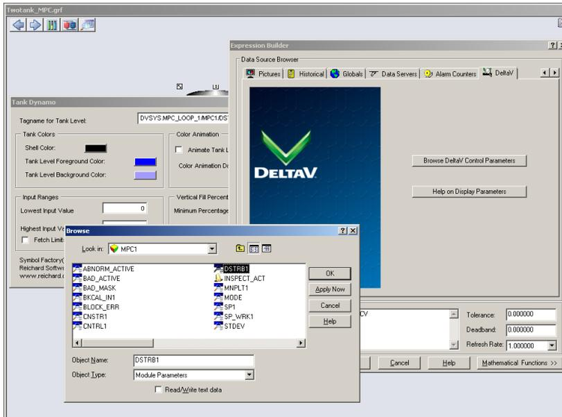
Figure 4.5 Linking level data to tank 1.
