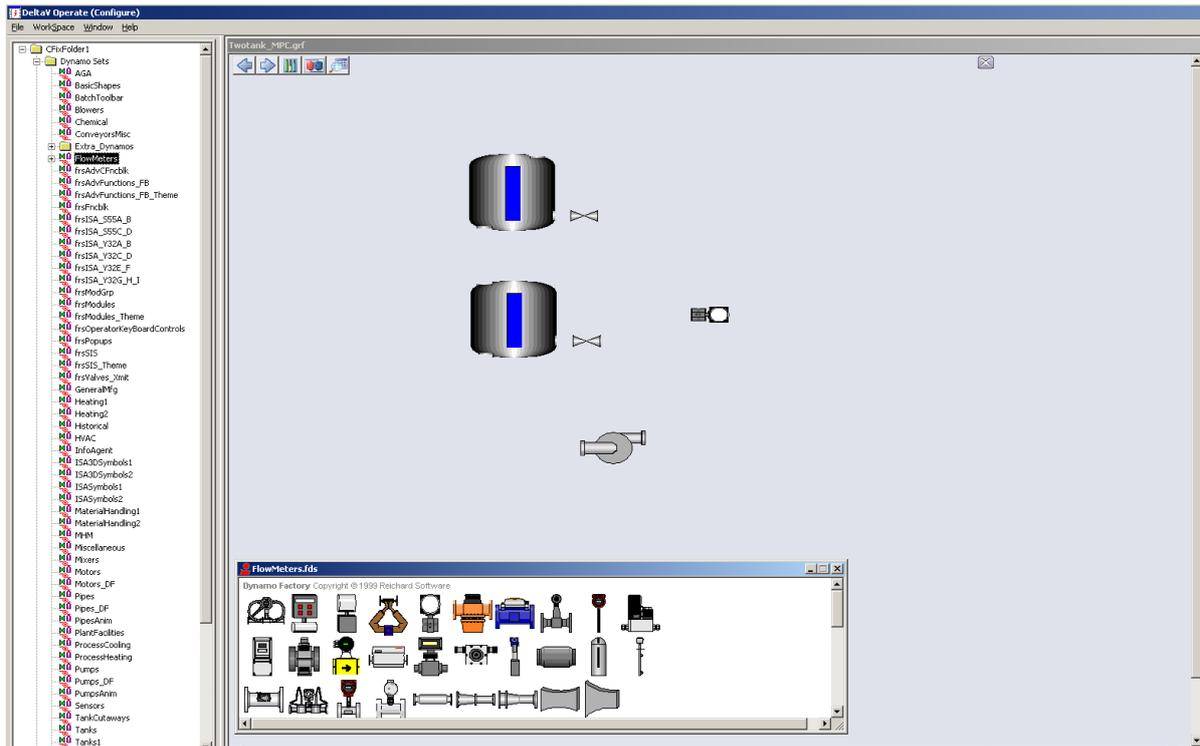
Figure 4.12 Adding a flow transmitter to the picture interface.
