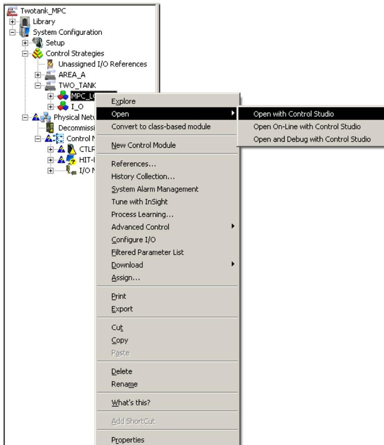
Figure 2.7 Open control module in Control Studio.
