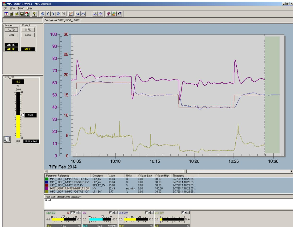
Figure 3.14 Testing the MPC controller in MPC Operate.
