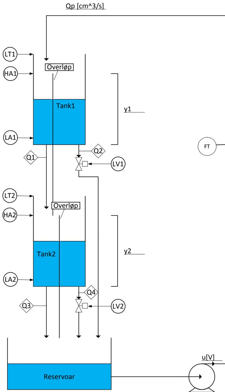
Figure 1.2 P&ID drawing of the Two-Tank system.
