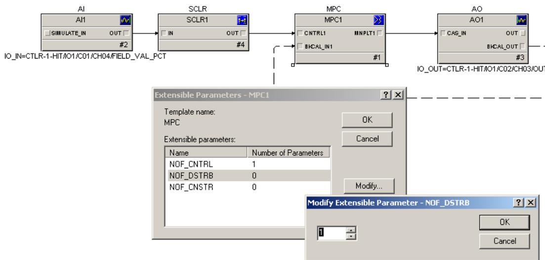
Figure 2.10 Adding constraint and disturbance variables.
