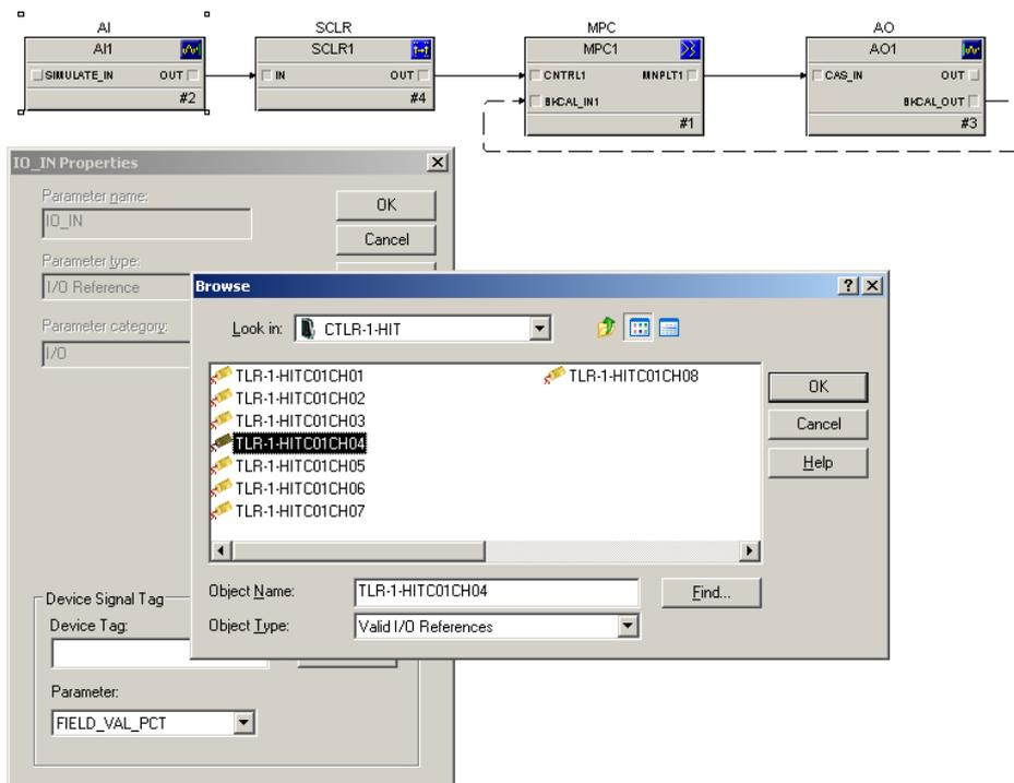
Figure 2.9 Assign I/O to Signal Tag.
