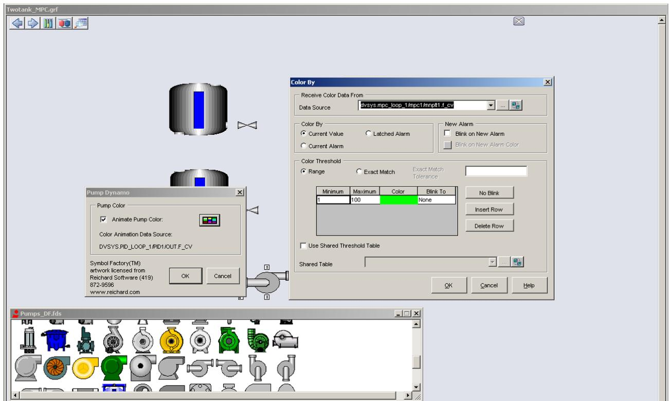
Figure 4.11 Linking manipulated variable data to the pump and adding animation color.
