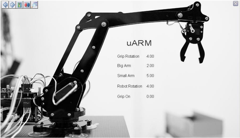
Figure 14. The DeltaV user interface, where the operator is able to change by activating the the control variables for the uArm.
