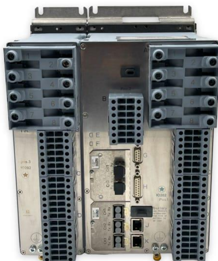
Figure 6 - Example of rear side of IED, showing a SIPROTEC 5 digital protection relay with multiple electronic interfaces [10].
