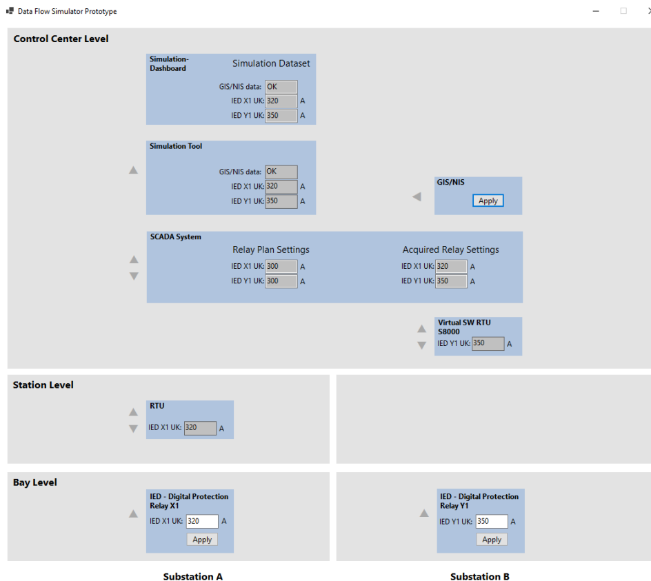
Figure 10 - Data-flow simulator prototype GUI showing the main elements and data-flow in the dynamic relay settings scope. The GUI is inspired by the architecture shown in figure 1.
