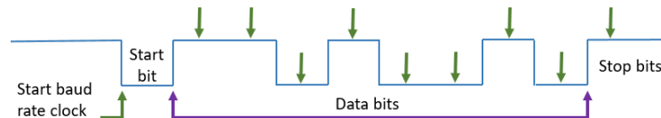
Figure 1.4: The transmission of the bits in asynchronous serial communication. It will start with a start bit, then the data bits, and a stop bit at the end.
