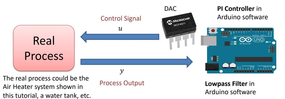
Arduino has Analog Input pins so reading the process value is no problem
